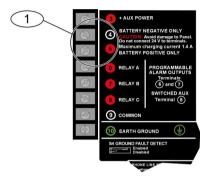
Figure 4.1: Battery Terminals
